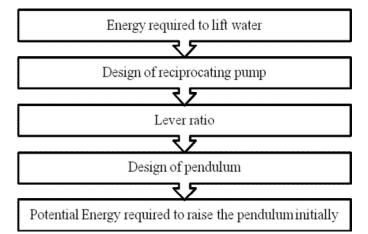
The above flowchart shows the steps involved in the design of whole system. In this process first the output required to lift the water from a particular height is calculated. Based on this output the pump was designed and then the input required by the system.
