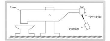
Figure 3: Conceptual Design of Two-Stage Oscillator
